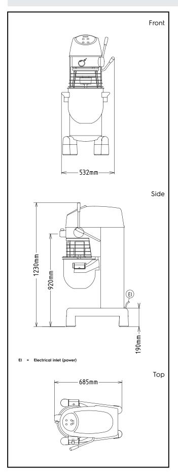
**Electric** Supply voltage: 200-240/380-415 V/3 ph/50 600250 (XBM20AB3) 200-220/380-440 V/3 ph/60 600252 (XBM20AB36) Capacity: Performance (up to): 6 kg/Cycle Capacity: 20 litres
